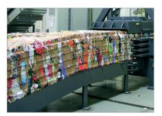
**Strapping** Fully automatic 5-fold strapping for optimal bale result also with expansive materials.
