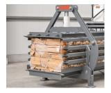
Suitable for compressing paper, cardboard, shredded material and plastic film
