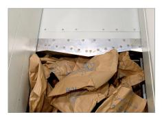
**Automatic operation** Control of the pressing process via light barrier.
