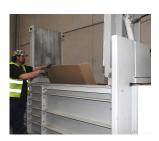
Especially large loading aperture for bulky materials
