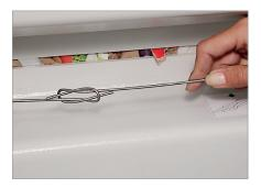
**Strapping** Manual bale strapping with Quick-link wire.
