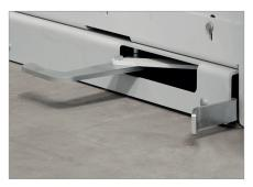
Pallet locking mechanism Pallet locking mechanism for safe bale removal.
