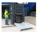
Safeguarding of the operating area with protective grid for maximum operator safety
