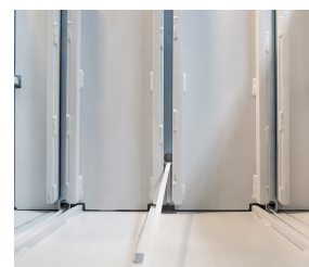
Compaction against counterplate by horizontal moving press ram
